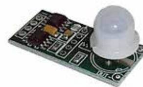
*The electronic device is designed to turn the LEDs on and off thanks to a Motion Sensor. The sensor detects the movements with 120° angle and 3 meter apart. Without motion the device turns off the LED after 30 seconds. Wired with 50 cm in/out.*
