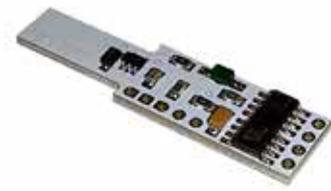
*The electronic device is designed to turn the LEDs on and off thanks to a Touch Sensor. Wired with 50 cm in/out.*
