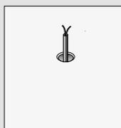
*As first step fix outer casing during realization of the block and thread wire through electric tube up to the recessed box.*
