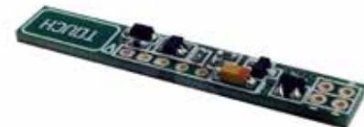
*The electronic device is designed to turn the LEDs on and off thanks to a Touch Sensor. Wired with 50 cm in/out.*
